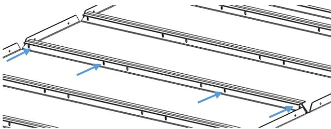
Figure 5: Bolting Panel-to-Panel
