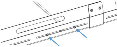
Figure 13: Side Rail Attachment
